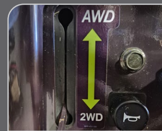
SELECTABLE DIFF LOCK AND 4WD CONTROLS.
