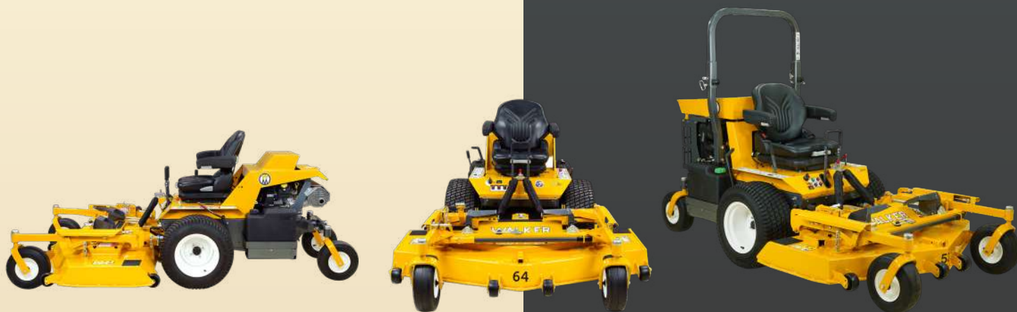
Pictured: H38i (left, middle) with a 64" (163 cm) rear discharge deck and H24d (right) with a 52" (132 cm) rear discharge deck.
