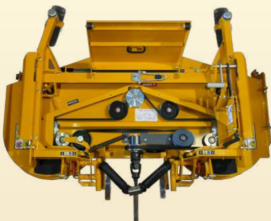
DS60-3 Belt Drive Deck (top cover removed)
