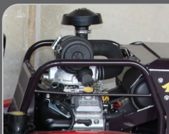
23HP V-TWIN VANGUARD ENGINE.
