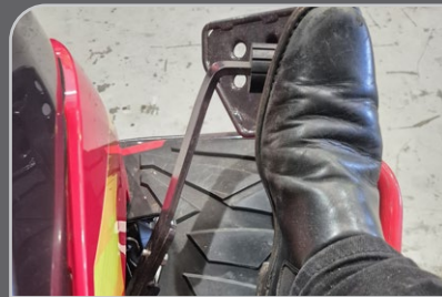
FOOT PEDAL HEAL/TOE FORWARD REVERSE.
